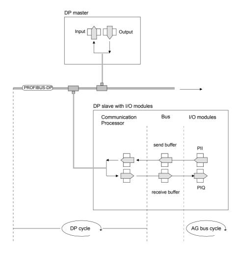
PII: process image of the inputs PIQ: process image of the outputs
